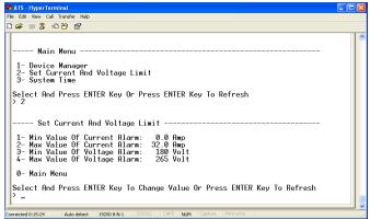
Enter corresponding number to Re-define the item that user want to change, select 1 to set the minimum value of current to alarm; select 2 to set the maximum value of current to alarm; select 3 to set the minimum value of voltage to alarm; select 4 to set the maximum value of voltage to alarm. For instance, If user want to change the value of the minimum current to alarm, enter 1 then press Enter to enter the interface as below:
