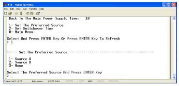
12.1. Enter the corresponding code, for instance: Enter 1 then press Enter to select input A as the preferred power input. The interface will return to Device Manager interface. See the below window: Preferred Source: Source A means that input A was select as the primary power source
