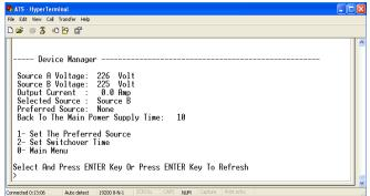
13. Set the Re-transfer time, the path are: Main Menu=>1 (Device Manager) =>2 (Set Switchover Time) enter the value preferred then press Enter. The Re-transfer time ranges from 10 to 60 seconds. The ATS will transfer to the preferred input power after defined time when user give the order to transfer or the preferred input line recover from power failure.
