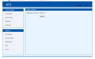
Note: Make sure there is no power failure, no internet disconnection, and no operation on the web interface during restart, If the device is directly connected to PC, the local connection will disconnected and connected automatically.
